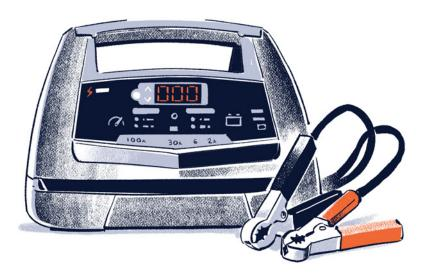
Trickle chargers come with downsides as well. Cheap ones can overcharge the battery and cause fires. Check the internet for horror stories and photos if you don't believe it. Trickle chargers without internal float controls also can ruin batteries when left on for a long time, thus killing the thing that they are meant to be saving.
