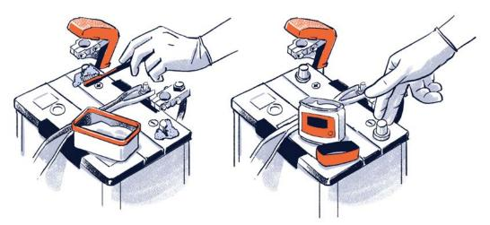
**Using a battery/trickle charger:** A trickle charger provides a steady low-amperage charge to the battery; a more sophisticated float charger senses when the battery is starting to discharge, then applies a charge to the battery until it is topped up again, at which point it switches off. A discharged battery can freeze, so either keep it on a charger when stored in winter or remove the battery and store inside.
