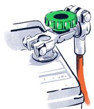
a shocking amount of power and can easily start fires if metal bits are touching each other in the right way. Some people have had good luck with the inexpensive screw-type disconnectors—the kind typically with a green knob—yet others prefer using marine-rated shutoffs.
