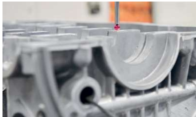
Quality control using 3D measuring probes on the processed individual part.
