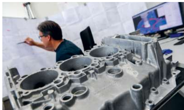
Processing of the poorly legible drawing data and comparison of the digital data of the motorsport engine.
