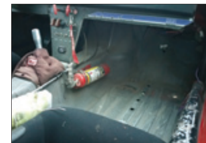
Sp1 holes in firewall and floor (top photo). An cracked exhaust manifold had exhaust entering the driver's compartment
