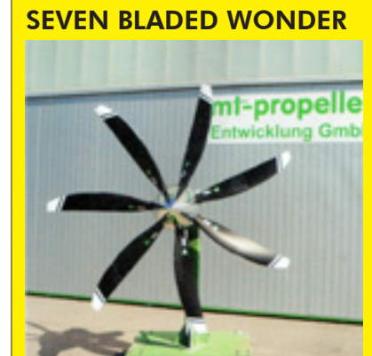
From October's Sport Aviation, an amazing breakthrough in propeller design. Seven (and soon nine) blades. Less noise, lower rpm gearboxes, improved takeoff and climb and improved performance
