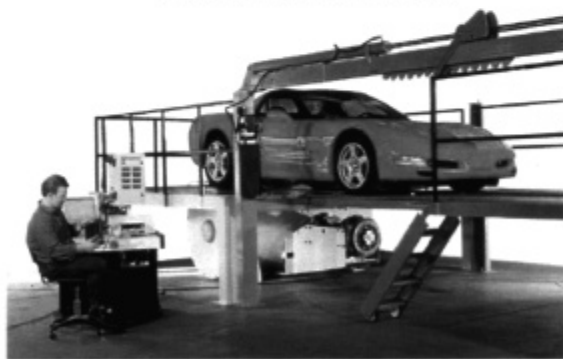
actual Speed Lab dyno installation is in-ground
