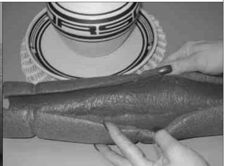
The view of the inside reveals a distinct splitting of the foam.
