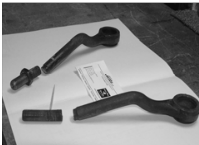
Fig. 6 Broken tie rods from the same car
