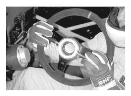
T C Racing's quick release mechanism makes it easy to insert and remove the steering wheel from the hub. Simply pull the twin pins. Direct bolt-on installation to Momo, Sparco and other steering wheels.
