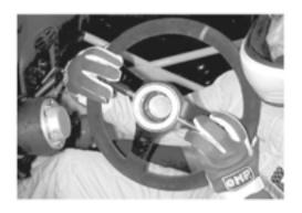
T C Racing's quick release mechanism makes it easy to insert and remove the steering wheel from the hub. Simply pull the twin pins. Direct bolt-on installation to Momo, Sparco and other steering wheels.
