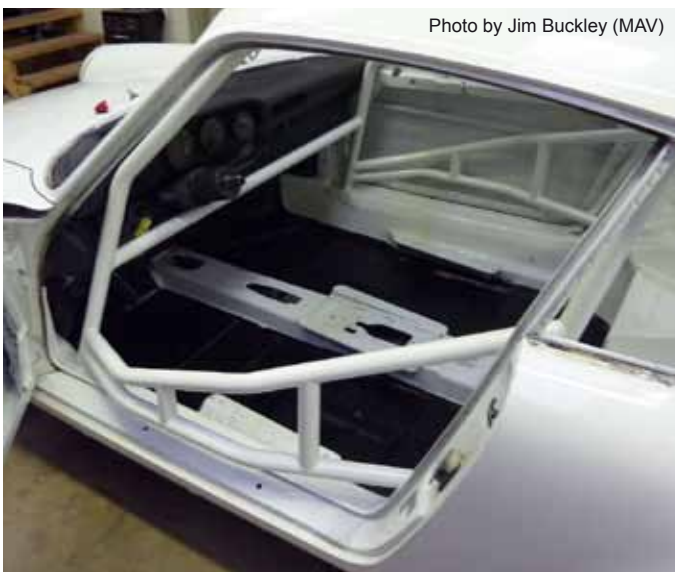
Proper stock class interior removal - cleaned and painted
