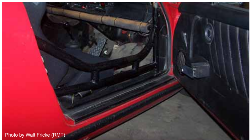
Double door bars with two vertical braces and minimal door panel removal
