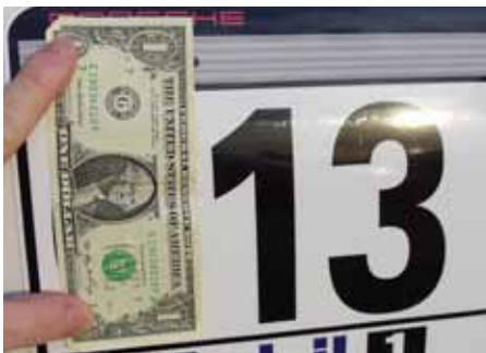
Figure 2: Car number failing the dollar bill minimum stroke test
