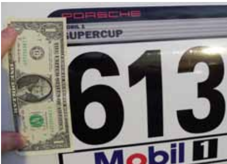
Figure 1: Car number failing the dollar bill minimum height test
