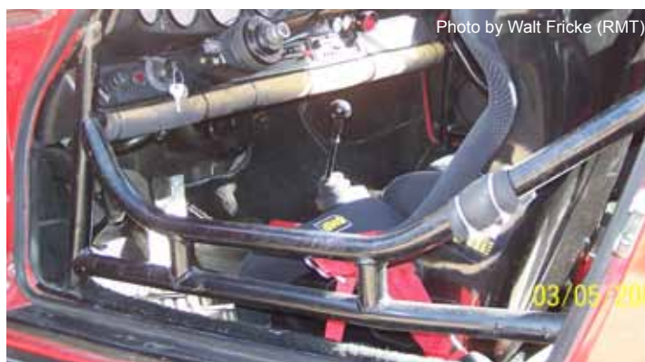
Double door bars with two vertical braces
